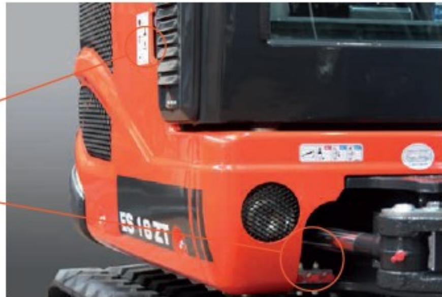
The battery, fuses and hydraulic oil top up can be reached through special compartments on the front of the drivers location.
