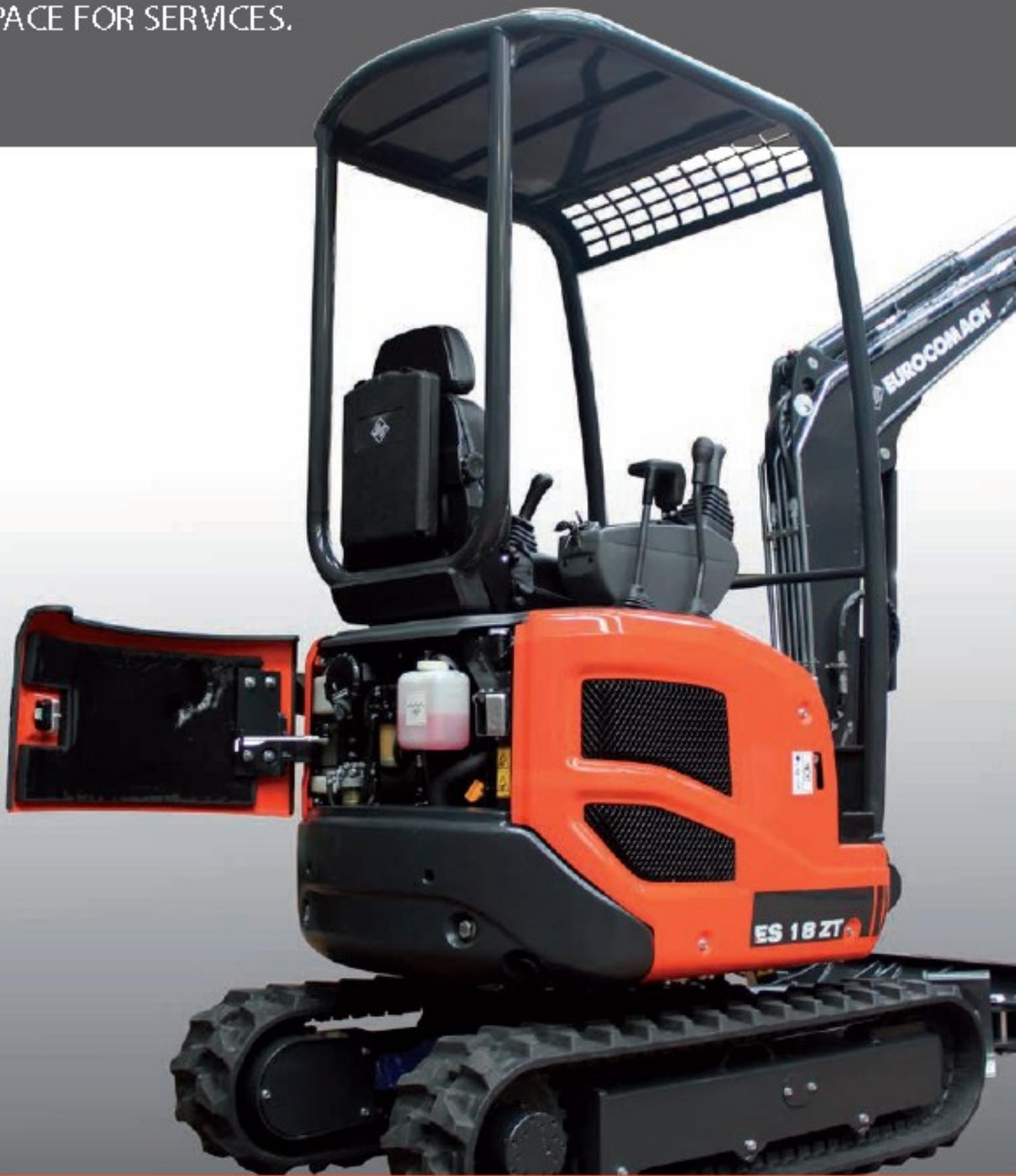
The rear engine compartment offers easy access to all filters on the heat engine (fuel, oil and air) in addition to easy topping up of cooling liquid and motor oil.
