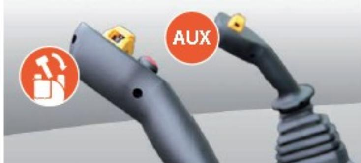
Auxiliary hydraulic system hookup with Proportional electrohydraulic control on the joystick
