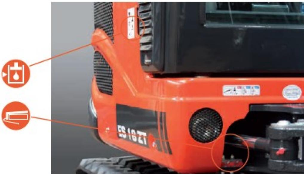
The battery, fuses and hydraulic oil top up can be reached through special compartments on the front of the drivers location.
