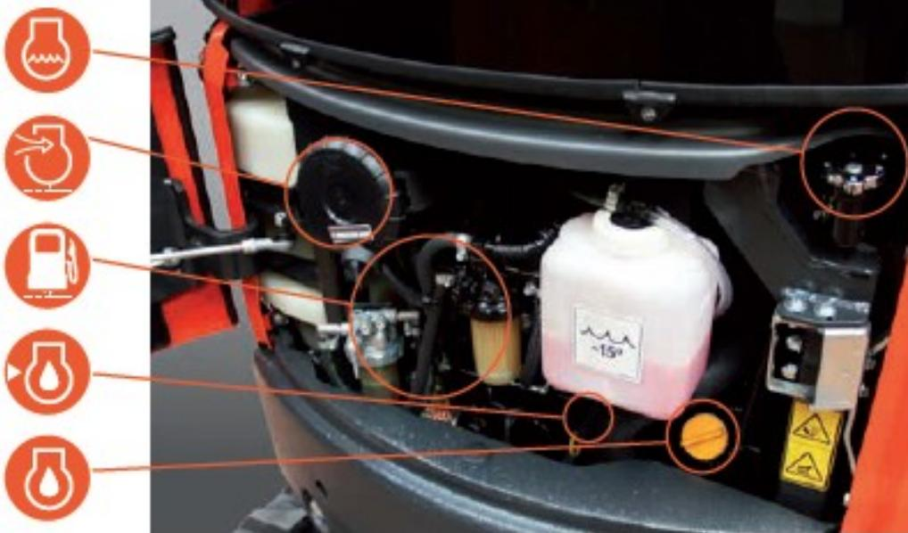
All access points for daily checks and for routine maintenance are easily accessible and concentrated in defined areas, optimizing machine downtime.
