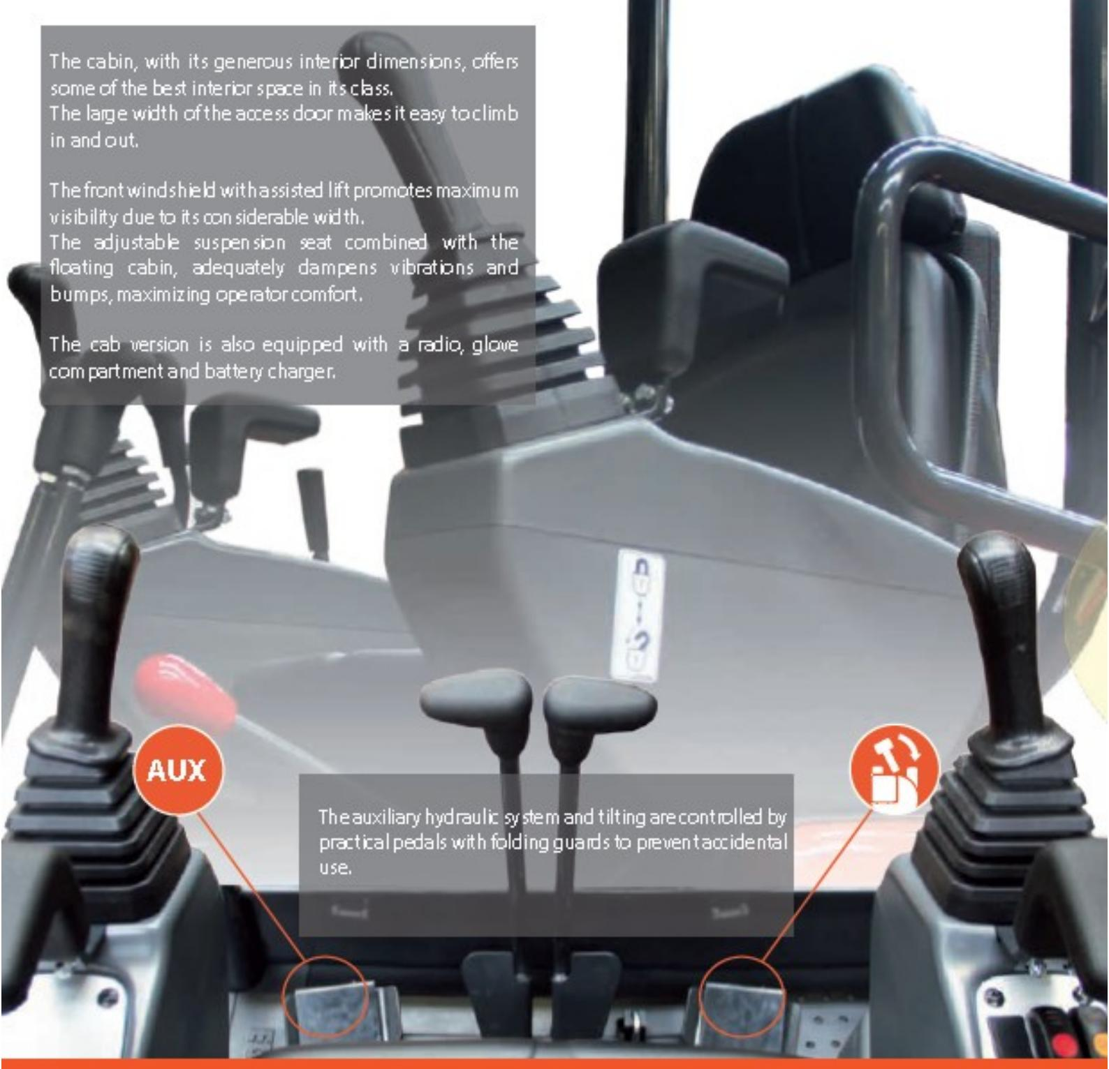
The auxiliary hydraulic system and tilting are controlled by practical pedals with folding guards to prevent accidental use.
