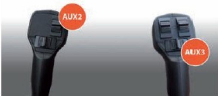
Electro-hydraulic proportional potentiometer to act the hydraulic system on both Joysticks
