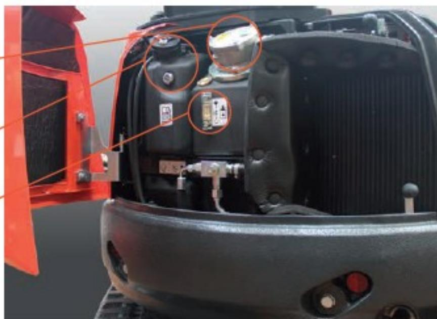
Services related to the heat engine are easily reached through a wide opening and the side compartment. All the filters (fuel, oil and air) in addition to checking and topping up the engine oil, are easily identified on the side.
