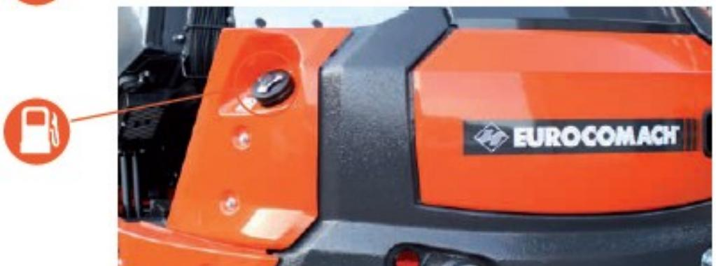
The rear compartment allows quick access to the electronic pump to refill the fuel and to the hydraulic distributor.
