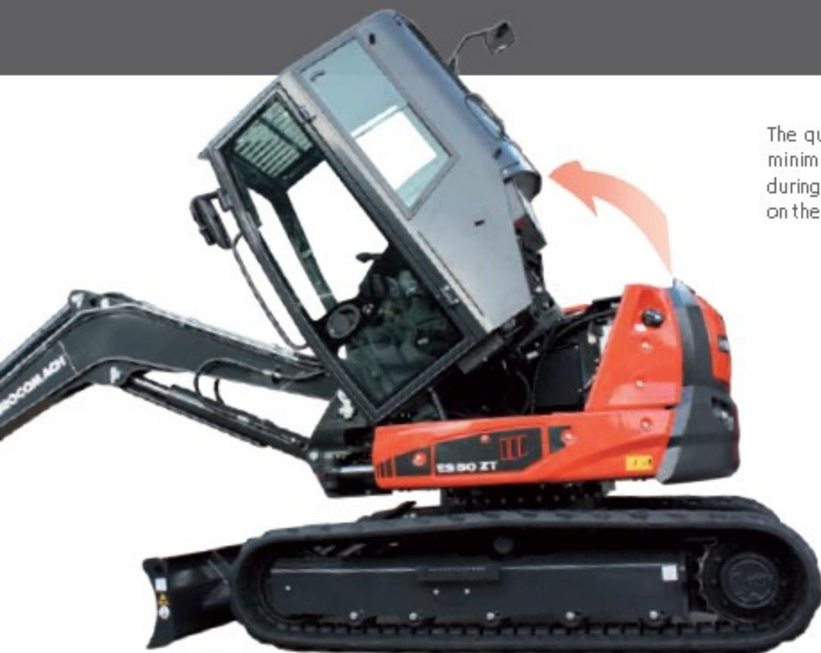
The quick and practical cab tipping minimizes machine down time during extraordinary maintenance on the hydraulic system.
