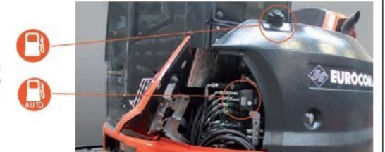
Services related to the heat engine are easily reached through a wide opening and the side compartment. All the filters (fuel, oil and air) in addition to checking and topping up the engine oil, are easily identified on the side.
